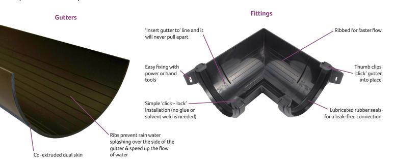
FlowPlumb Systems™ Rainwater Gutters are co-extruded for longer life, higher weather durability and a high gloss finish. The "dual skin" protects the gutter from UV bleaching and adds a touch exterior layer.
